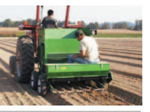
*Figure 2.* Sowing oak acorns from large hopper on the front of the planter and wheat seeds from small hopper on the back. (Planter built by Jack Seifert and crew.)
