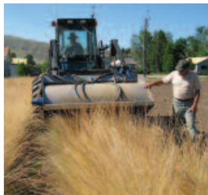
Figure 4. The modified seed stripper harvesting Arizona fescue at Lucky Peak Nursery.
