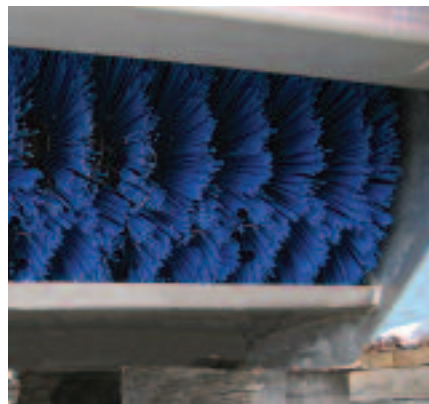
Figure 3. The modified design uses a cartridge system where convoluted wafers stack together to form the brush. Open voids and the wedging pattern of the bristles help pull seeds from the seed heads of grass and forb plants.
